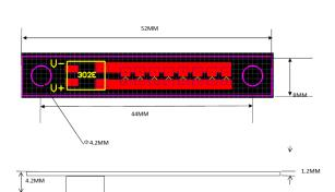
The MinEM is a miniature dedicated emergency LED strip which is designed for auxiliary emergency applications, where the mains light source cannot be converted to emergency.
