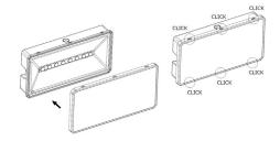
4 - Return and click the geartray to its operational position. Replace the cover, making sure there is a click at all six points to maintain IP rating.
