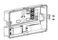
3 - Connect the supplies and, where required DALI bus. Once power is assured, connect the battery connector. Ensure that the cable clamp is tightened.
