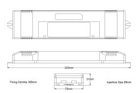
T2N/2/SP85/R Prated - 4.3W Irated - 85-14mA Voltage Range 50 - 300 Volts Open Circuit Voltage (U-OUT) = 350 Volts
