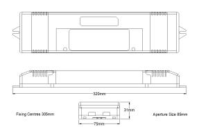
The TLP/2/SP85/R is supplied as a remote conversion kit designed to be mounted adjacent to the luminaire, where room inside the fitting is limited. This unit offers a higher output which is more suitable for higher power luminaires.
