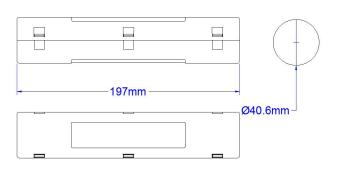
The S/CBH range is supplied as a complete ceiling recess emergency pack to power one of a range of dedicated emergency LEDs from a central battery or static inverter system.
