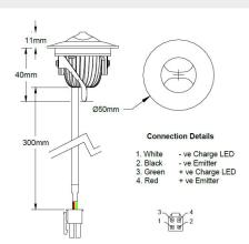
The LED/40/CO is a discrete emergency LED which is designed for ceiling recess applications along corridors. The bezel has a diameter of 50mm and the cut out required is 43mm.
